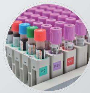
The special tube racks utilize different barcodes to differentiate specific usages, such as "QC", "Slide making & staining only" and "RET test only". The special tube racks can carry the tubes to perform these specific functions in the simplest way.
