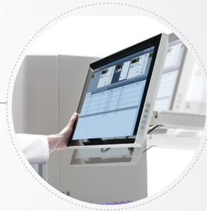
The touch screen is the "brain" of CAL 8000. It optimizes the distribution of workload between each BC-6800 unit and decides which sample requires a blood smear. It displays the status of each BC-6800 or SC-120 installed on CAL 8000 as well as the volume of balance reagent. This intuitive software can tell the users all necessary information of CAL 8000 at any given time. Consequently, the users will spend less time operating CAL 8000 and arrange their working schedule better.
