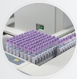
The stock yard can hold up to 300 sample tubes at a time. From here the users can select the sample tubes which need further analysis.
