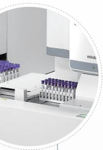
The CAL 8000 can automatically distribute the samples with "Repeat", "Rerun" and "Reflex" criteria which are pre-defined by users.
